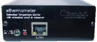
The Ethermometer monitors temperatures in equipment rooms, rack rooms, unoccupied homes, transmitter or remote equipment sites, wherever you need to monitor and report temperature!
