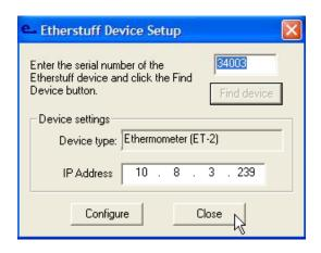
If your LAN supports DHCP, your ET2 will have a meaningful IP address already in the IP address field of Etherset; write it down and click close. If your LAN doesn't support DHCP or you wish to assign a Static IP to your ethermometer, enter the static IP in the IP address field and click configure, then close.
