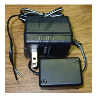
The PF-1 Power Failure monitor.
